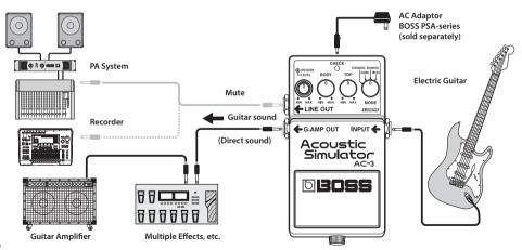
The following shows the correspondence between output jack connection status and the sound output.
