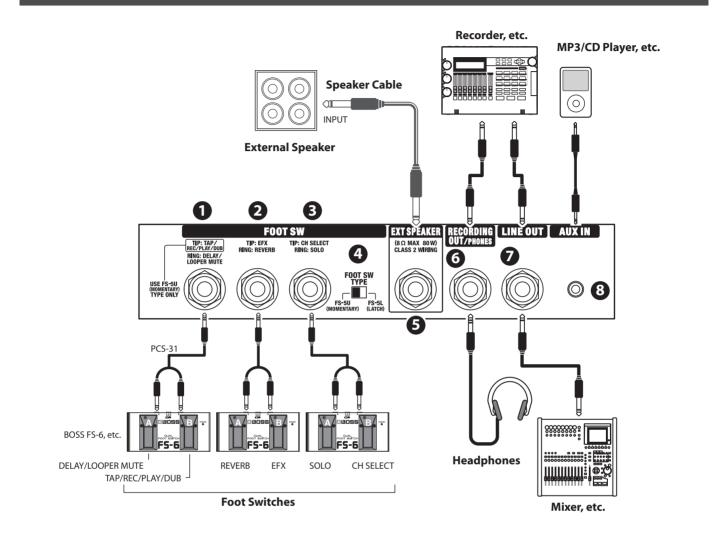
\* To prevent malfunction and/or damage to speakers or other devices, always turn down the volume, and turn off the power on all devices before making any connections.
