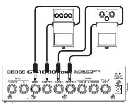
The sound that is input to SEND/RETURN within the effect chain will be output to the SEND jack. The sound that is input via the RETURN jack will be input to SEND/RETURN within the effect chain.
