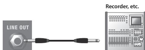
You can use this in conjunction with an external PA system, or to record your performance via direct line while monitoring the sound from the KATANA's speaker.
