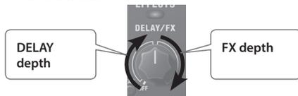
\* Either DELAY or FX is selected depending on the position of the knob.
