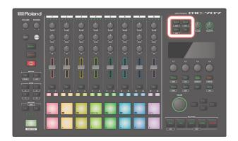
By pressing one of the [REVERB] [DELAY] [MULTI] buttons you can change the target that is operated by the knobs.
