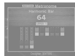
Lets you pull out all of the harmonic bars using a single knob. If you continue turning the knob after all of the harmonic bars are pulled out, the rotary effect will switch to the fast state (p. 22).
