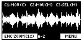
3. **Decide on where to add the marker by using the [CTRL 1] knob, and then press the [MARK] button.**
