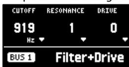
You can also access the effect sub-parameters by holding down the [VALUE] knob and operating the knobs.
