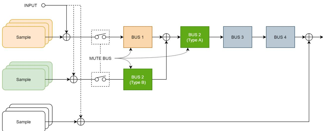
Also, the diagram below shows how the audio outputted from this unit changes when you turn MUTE BUS on/off.
