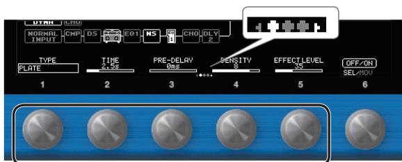
Use the PAGE [◀] [▶] buttons to switch between the parameters that you want to edit. The current page is indicated in the lower center of the screen.
