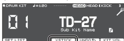
When playing using a pad that supports digital connection and cross-stick technique (such as the PD-140DS)
