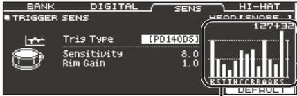
Velocity meter (Indicates the force (velocity) of the strike.)
