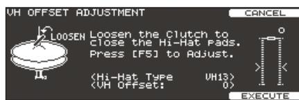
6. Loosen the clutch screw of the top hi-hat and let it sit on the bottom hi-hat.
