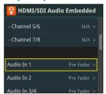
5. Use the [VALUE] knob to select "Dry", "Pre Fader", or "Post Fader", and then press the [VALUE] knob.
