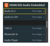
3. Use the [VALUE] knob to select the input audio you wish to assign to the channel, and press the [VALUE] knob.
