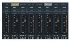
2. Use the [VALUE] knob to select the tab at the top of the screen, and press the [VALUE] knob.
